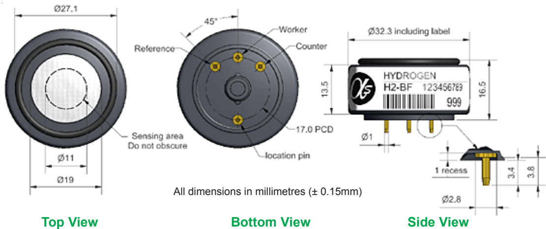
Figure 1 H2-BF Schematic Diagram
